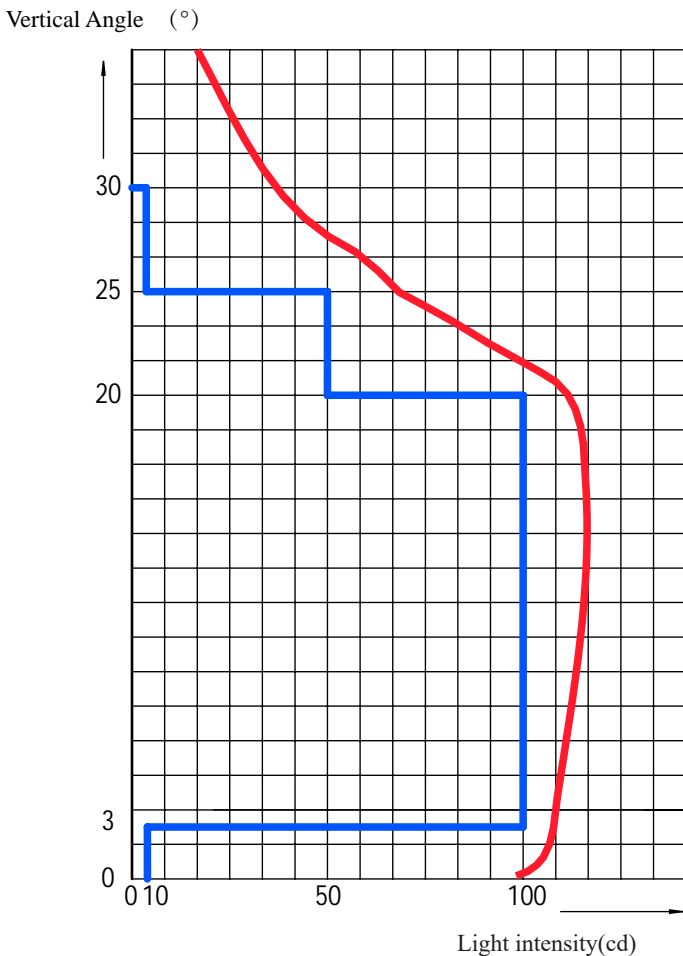
LED Inset Aiming Point Light (white), AC-137-CA chapter 5.2.1.6
